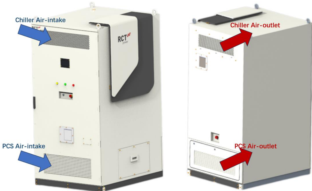
Fig. 4-5 Ventilation Design
